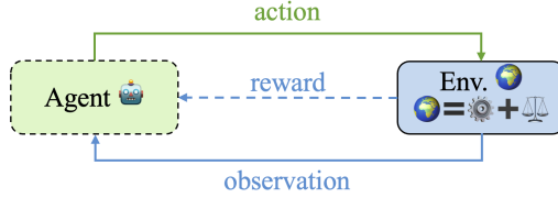
Figure 4: Pictorial illustration of Online RL: an agent actively interacts with the environment, which is composed of the dynamics model that controls transition, and the reward model that provides feedback.
